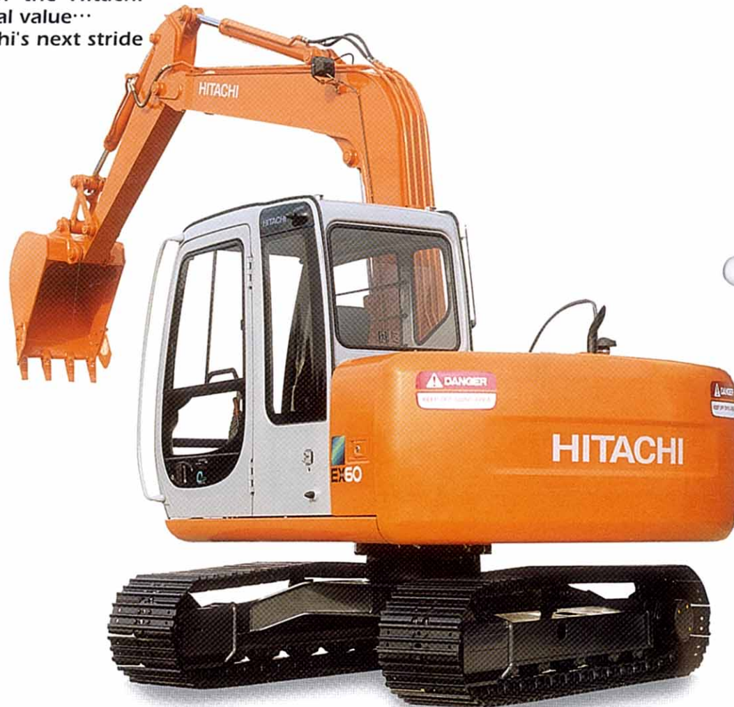
The EX60-s fitted with 3.72m (12'2") boom, 1.62m (5'4") arm and 0.28 m 3 (0.37 yd 3 ) bucket
